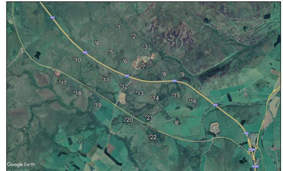
Figure 1 Wind development turbine layout
